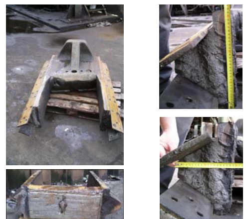
Damaged cutting slide of a shredder machine
