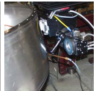
Keyhole welding on large sheet metal parts
