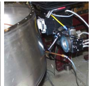
Keyhole welding on large sheet metal parts
