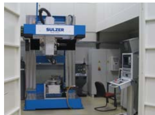
1.5 kW Fiber-Laser system 5+2 CNC-axes X-Y-Z 0.5 x 0.5 x 0.7 m B,C,D,E ±180°,360°,360°,±90° On-site operation possible
