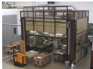
2 kW CO 2 -Laser system Gantry robot, 6 CNC-axes X-Y-Z 2.7 x 1.8 x 0.9 m A,B,C 360°,±90°,360° Integrated digitizing system
