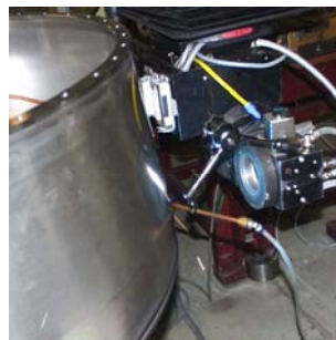
Keyhole welding on large sheet metal structures
