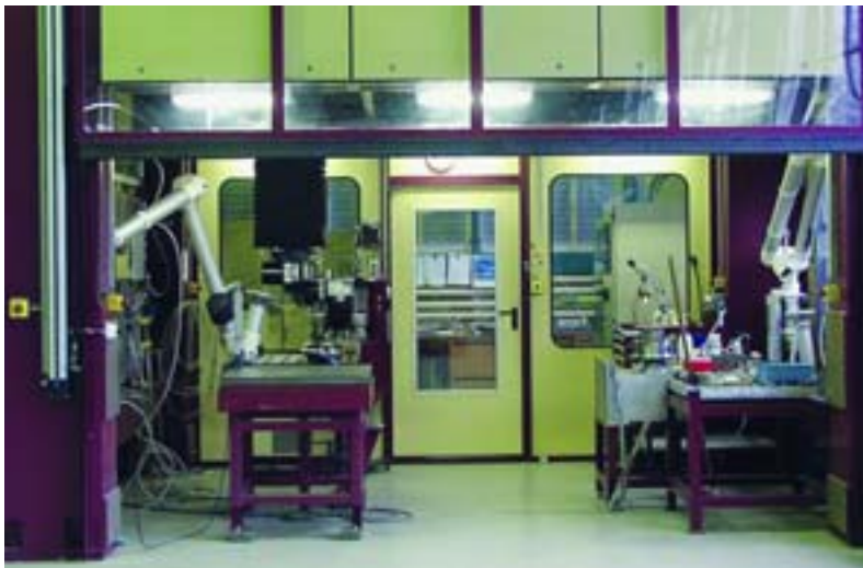
1 The laser welding system from Sulzer Innotec consists of a 2 kW CO 2 laser and a six-axis portal robot with a working space of 2.7 × 1.8 × 0.9 m.
