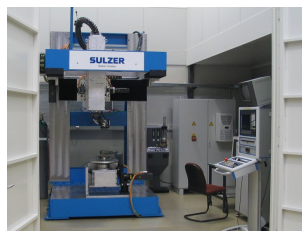
1.5 kW Fiber-Laser system 5+2 CNC-axes X-Y-Z 0.5 x 0.5 x 0.7 m B,C,D,E ±180°,360°,360°,±90° On-site operation possible
