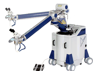
150 W Nd:YAG-Laser system Peak pulse power 10 kW Boom range 1.2 m Hand operated On-site operation possible
