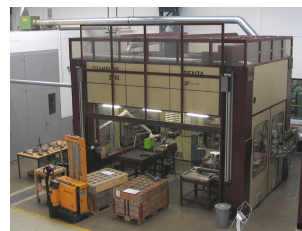
2 kW CO 2 -Laser system Gantry robot, 6 CNC-axes X-Y-Z 2.7 x 1.8 x 0.9 m A,B,C 360°,±90°,360° Integrated digitizing system
