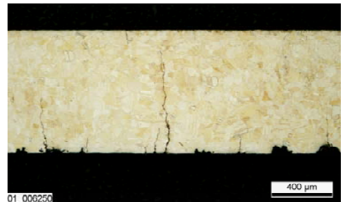
Stress corrosion cracking in a brass pipe taken from a heat exchanger
