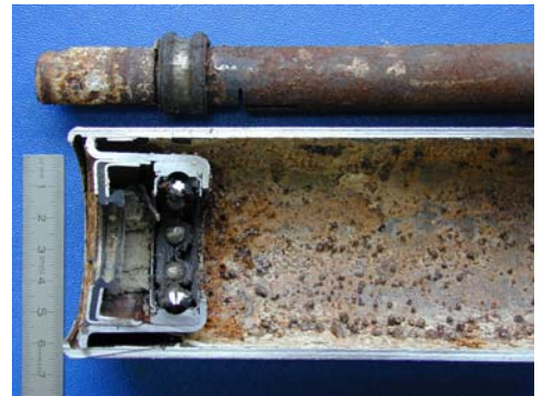
Corrosion damage on a conveyor belt roll-bearing
