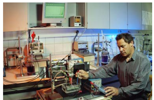
Tribo-corrosion test stand to determine electrochemical corrosion related data
