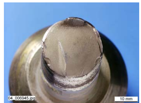
Fatigue fracture initiated by corrosion in a threaded bolt made of low alloy steel
