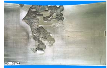
Defective bearing casing – was the right material used?
