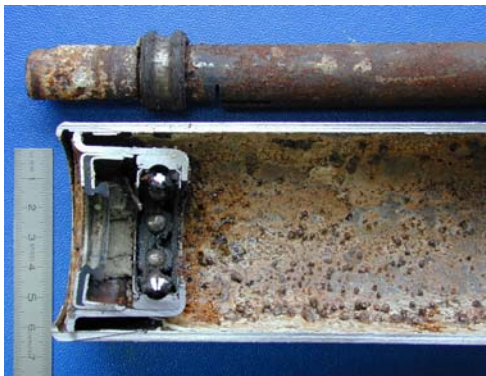
Corrosive damage in a roll bearing
