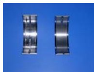
Quality assurance for bearing housing shells of white metal
