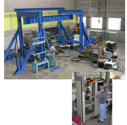
Various universal testing machines and a test platform allowing 100 m 3 volume for large-size test items
