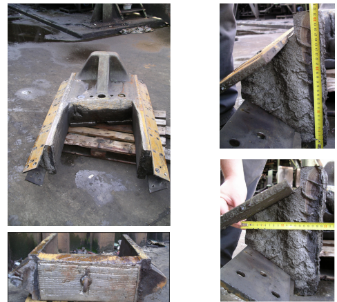
Damaged cutting slide of a shredder machine
