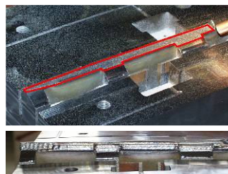
Knife edge weld build-up 200 x 10 x 10 mm
