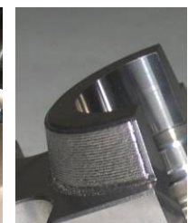
Precision build-up, 0.25 mm thickness
