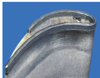
Blade tip welding
