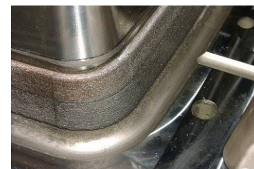
Correction of a curved geometry with undersize, 0.7 mm thickness
