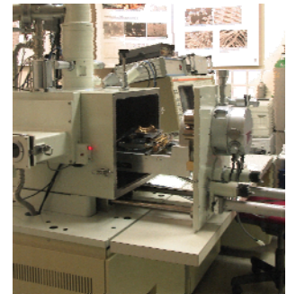
Our Jeol JSM-IC 848A Microscope The large sample chamber takes samples and components up to 200 diameter and 50mm height. The microscope is equipped with a state-of-the-art EDX for chemical analysis
