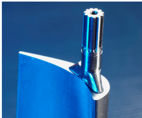
Gas turbine blade out of TiAl4VGr5 Optimization in manufacturing by integral design, 5-axes simultaneous milling from cylindrical stock material.
